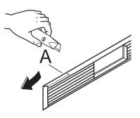
Re-install the grid to the base of the appliance by pushing the clasps (a) until they click.
